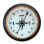
A barometer is a tool we meteorologists use to measure atmospheric pressure. That's a fancy way of saying we measure the weight of the air above us. When the atmospheric pressure is high, we can expect sunny, pleasant weather. When the atmospheric pressure is low, it's time to prepare for rain or snow. Barometers provide important "clues" meteorologists use to predict the weather.
