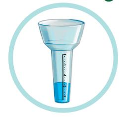
No weather station is complete without a rain gauge to measure the amount of rain that falls from the sky.
